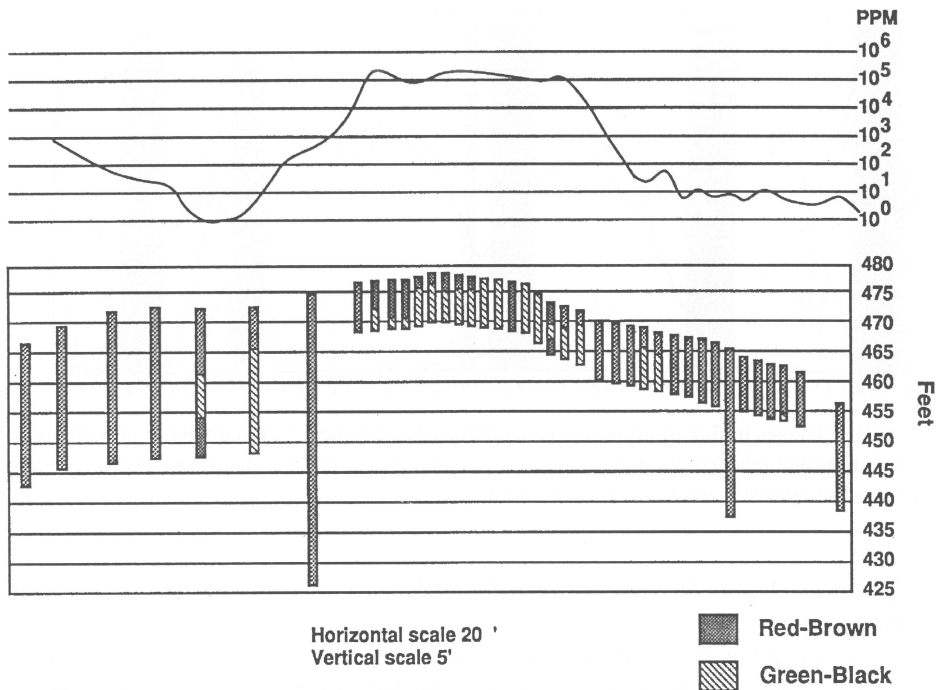
Fig. 5-11. Propane concentrations and soil colour of augered samples along a traverse of sample sites over an underground propane storage reservoir.
