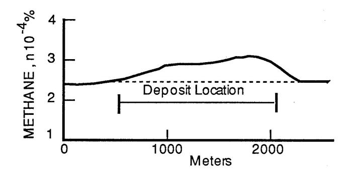
Fig. 5-14. Variations in methane concentration in air above a petroleum reservoir (reproduced with permission from Antropov et al., 1981).
