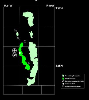
New production confirms predicted distance to production of 1 to 2 miles from non-productive test well.
